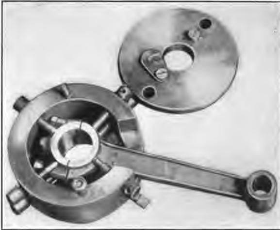
FIG. 33.—Holder used to prevent spreading.
